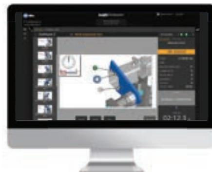
**1** Insight Centerpoint collects welding parameters such as voltage, amperage, wire-feed speed and gas flow.
