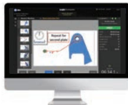
**1** Insight Centerpoint guides the welder through the fabrication process from pre-weld to post-weld in a standardized sequence.
