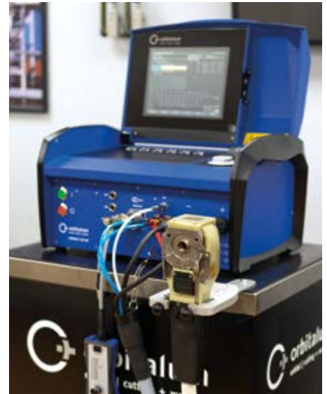
Arc Machines (AMI) Weld Head Connected to Orbitalum OM180 SmartWelder Power Supply
