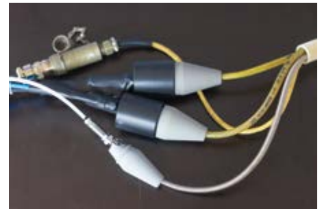
AMI Adapter Cable Connections feature protective sleeves
